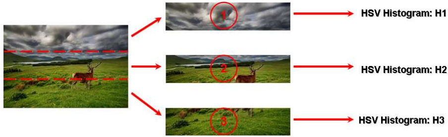
Figure 1: Dividing image on three horizontal segment to extract the histogram (HSV) of each part
