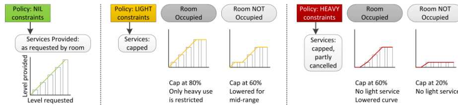
Fig. 4. Strategy for smart rooms: services provided given occupancy , need of room (level requested) for three energy saving policies (NIL, LIGHT, and HEAVY constraints)
