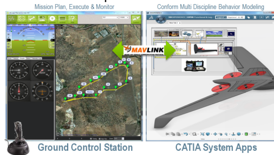
Fig 15. Ground Control Station and UAS communication
