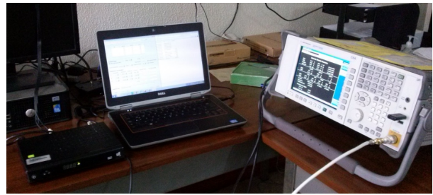
Fig. 7 Test scenario for transmission and reception of the ISDB-Tb signal
