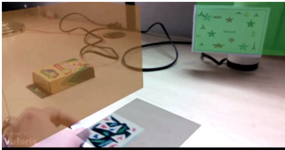
Fig. 3. MonitAR indicated the vacuum (top right) as the correct target object within the task and the crayon box (middle left) as the incorrect target object by highlighting the objects in green and red respectively. The hand (middle bottom) is highlighted in gray to indicate it is a recognized object.
