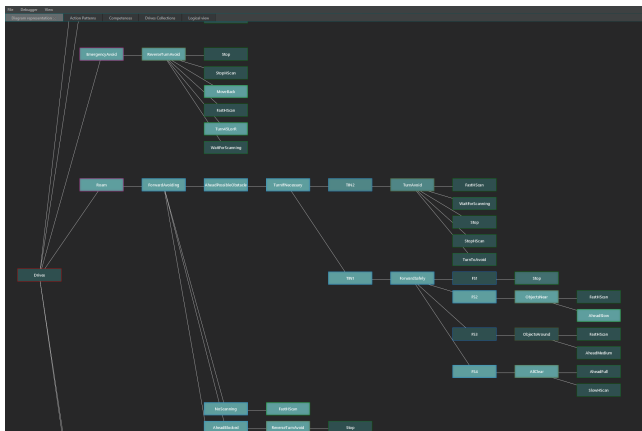
Figure 3: The ABOD3 Graphical Transparency Tool displaying a POSH plan in debugging mode. The highlighted elements are the ones recently called by the planner. The intensity of the glow indicates the number of recent calls. ABOD3 (used as an IDE for the entire hierarchical cycle) show everything ABOD3-AR uses parts only (2 levels only)
