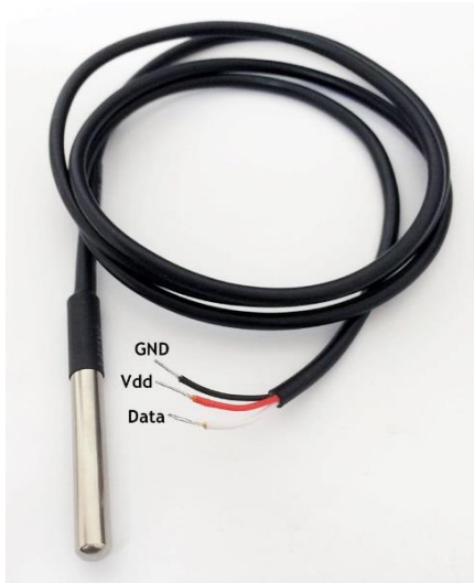
Figure 5. Waterproof temperature sensor DS18B20.
