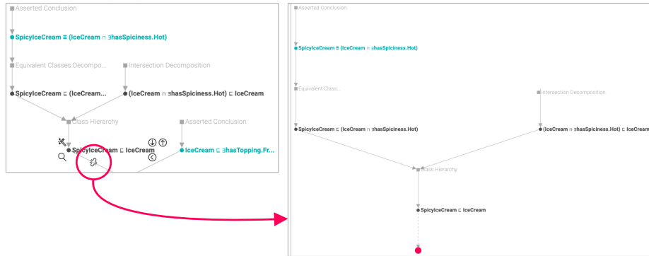
Fig. 5. Clicking on the delink icon next to the link in the left image isolates the sub-proof starting from this connection, which can be seen in the right image.
