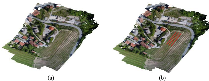
Fig. 5. (a) Extracted grapevine map from multiple UAV RGB images and (b) robot's trajectory between the lines (red color) of the vineyard.
