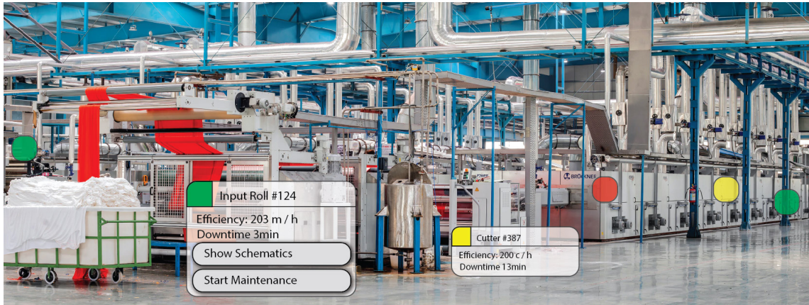
Fig. 2. Sketch of a smart factory maintenance scenario with different levels of scaled information shown to a user. While the worker maintains close proximity, more machine information and relevant interaction opportunities are available. The worker can see other machines in the distance with stack light indicators of their operational status.
