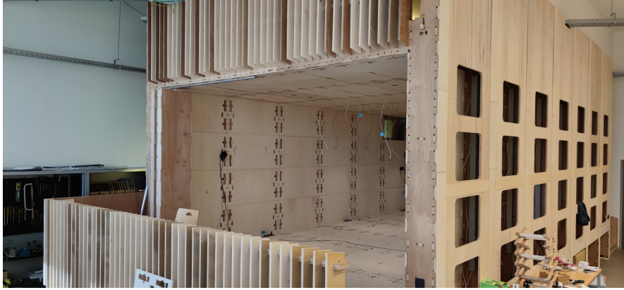
Figure 2: Techtile test environment, a 8 x 6 x 2.4 m wooden room.
