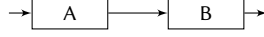
Figure 4: Task set \Gamma = \{\tau_A, \tau_B\} with a precedence relation between \tau_A and \tau_B
