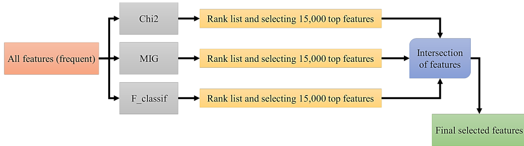
Figure 2: Steps involved in selecting the features using ensemble FS algorithm
