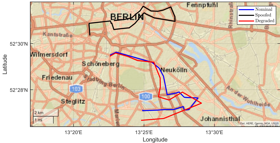
Figure 1: Examples of impact classification on different trajectories: in blue the authentic trajectory, in black a target trajectory for spoofing attack and in red a trajectory subject to PVT degradation.
