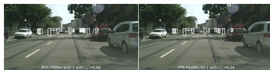
Figure 10: Inference results for BGC-HRNet-w32 (first run, best LAMR_T score with 8.8%) and FPN-ResNet50 (first run).
