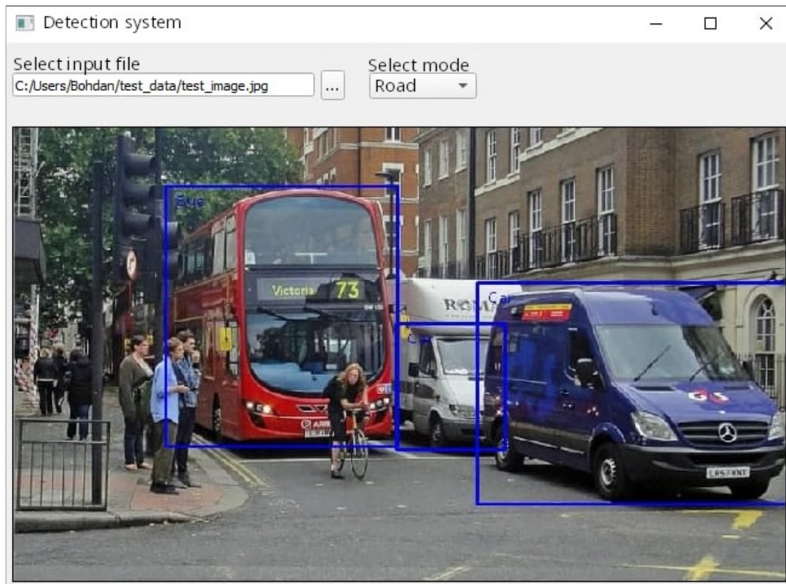
Figure 5: Object detection result with filtering (“road” mode applied)
