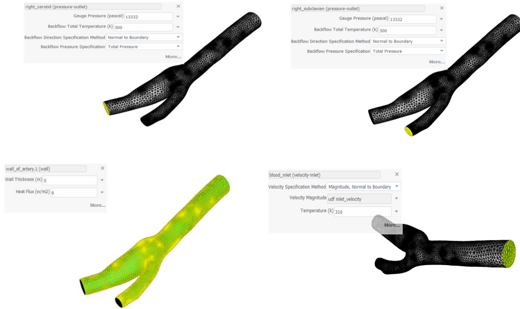
Figure 1: Coronary artery physical model with boundary conditions
