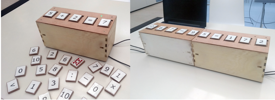
Figure 2: The figure presents two pictures, one representing one SMARTER 2.0 and math tiles (left side) and the other a possible scenario with two SMARTER modules joined horizontally (right side).
