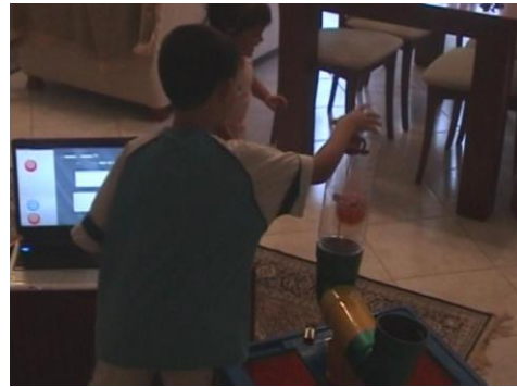
Figure 5. The kid plays the game ‘Tubes and Balls’ and NOESIS recognizes the color of the ball he is throwing into the tube using RFID coding. A complexity analysis is carried to identify pattern-locking and comprehension of the colors.
