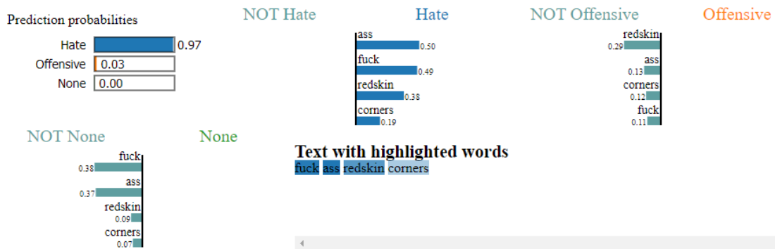
Figure 4: Hate Prediction by the BERT classification model along with explanations generated by the LIME pipeline
