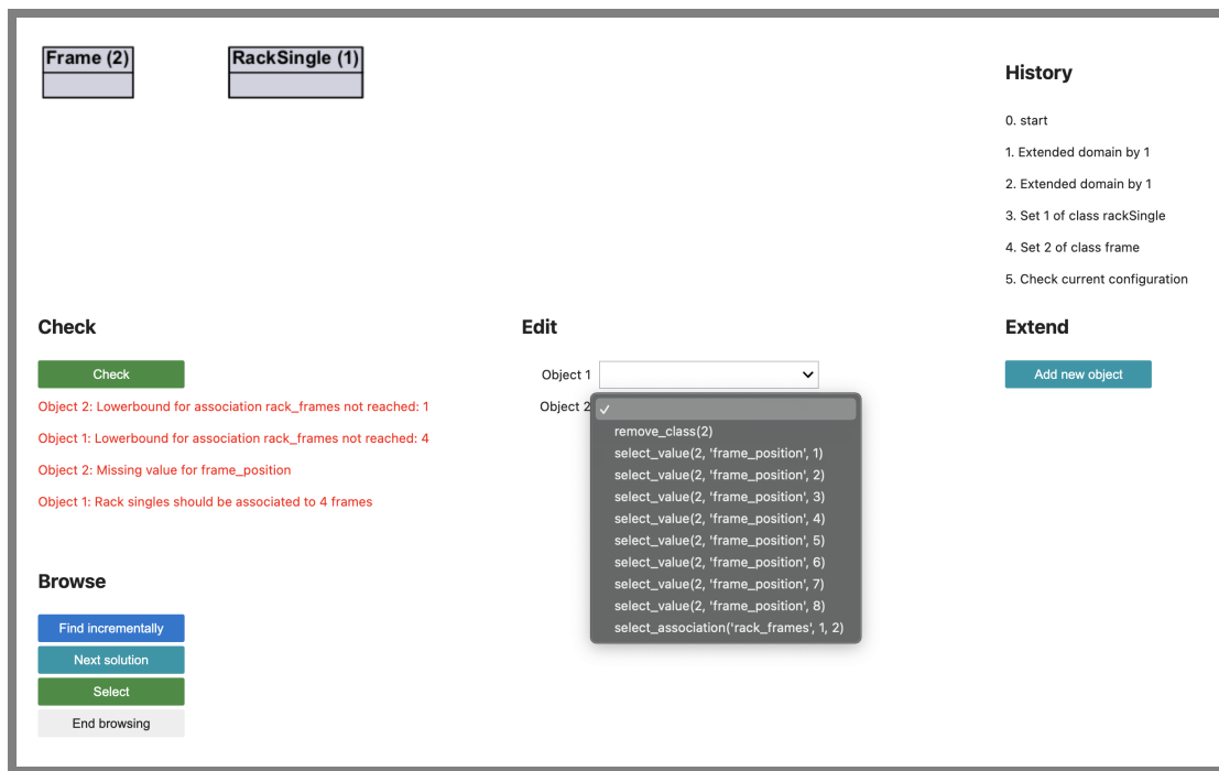
Figure 3: UI for interactive configuration generated with ipywidgets rendered in a Jupyter notebook.
