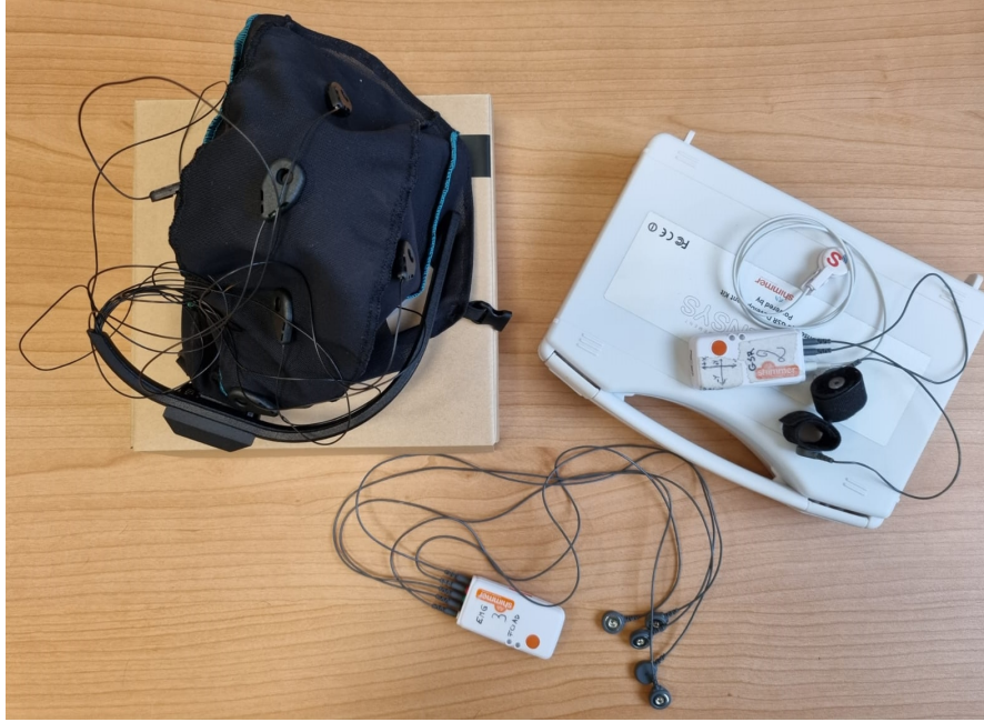
Figure 2: Physiological devices that will be used to record the subjects' physiological responses. From left to right, top to bottom: Unicorn, GSR/PPG device, and respiration device.
