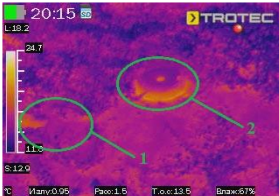
Figure 3. Thermal imaging at 20:15 on 09/08/2023 of anti-tank mines, where the number 1 and 2 indicate the place where the mine is buried and the mine on the surface, respectively.
