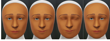
Figure 8: Four frames of an example Furhat robot emulation with different levels of smiles used as backchannels during the conversation in our user study.
