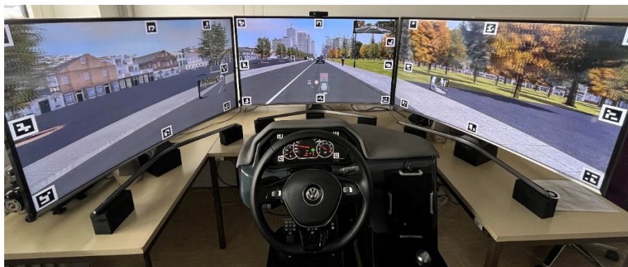
Figure 1: Driving simulator set-up used in the study
