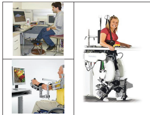
Figure 1: Successful examples of applied technologies for rehabilitation. They are all based on robots/exoskeletons and VR. Upper left: Rutgers Ankle, lower left Armeo® and right Lokomat®.
