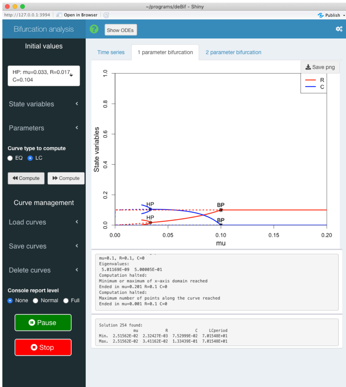
Figure 3.11: The 'bifurcation()' application during the computation of the curve of limit cycles (hence the 'Pause' and 'Stop' button) that originates from the Hopf bifurcation point (HP) to lower values of the bifurcation parameter. The maximum and minimum value of the state variables observed during the limit cycle are plotted as two separate curve sections originating from the Hopf bifurcation point (HP). The progress window reports the period of the limit cycle.
