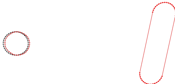
Figure 2.2-4: Examples of FTS FOV-areas projected on the earth's surface (a 36-polygon). The left depiction is for a computation while the IMC is "on" and the right depiction is for one with the IMC "off". Dark dots represent FOV-area before Ortho-correction, while red dots show after Ortho-correction. The right depiction shows a
