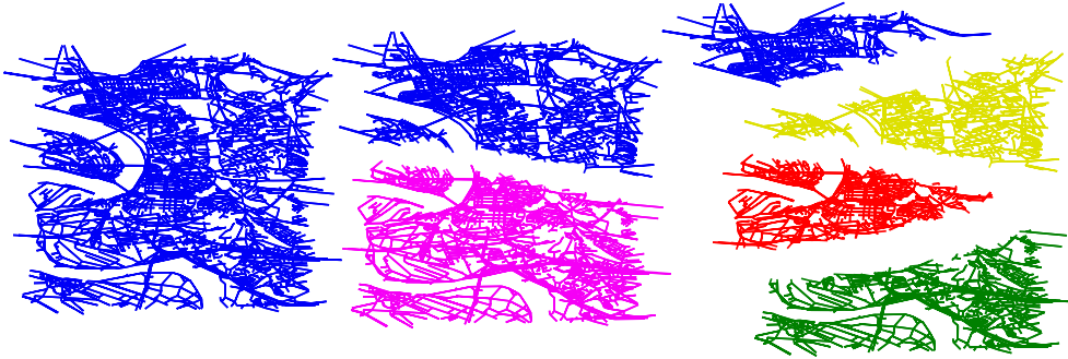
Figure 6.4: Map of Düsseldorf partitioned with KL-GM algorithm.
