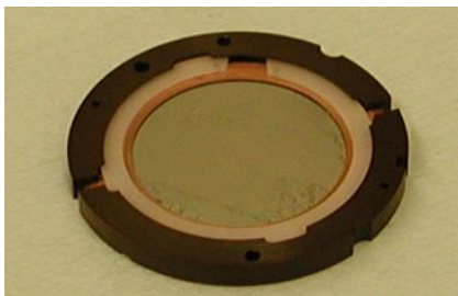
Fig 2. The cathode/target polyimide ring. The copper ring holding the mylar, can be seen beneath the delrin retaining ring.
