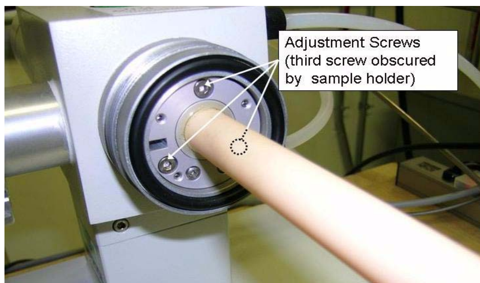
Figure 6. Close up view of sample holder adjustment screws.
