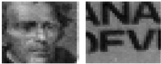
Fig. 16 Example images collected with image sensor ALOHAim2. President Jackson and ‘Analog Devices’ text. Images were collected with the sensor operating at 7.6 K events/s
