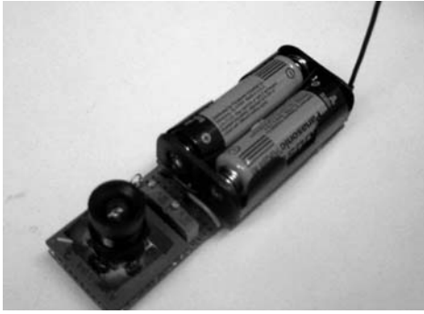
Fig. 1 ALOHA image sensor in a sensor network node
