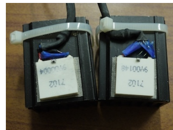
Figure 5: Peltier devices used (2 x 2cm 2 ), with black heatsinks.
