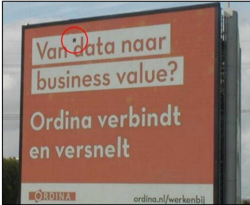
Figure 4 Example footage of billboard with broken LED tile
