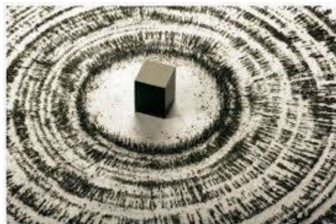
Figure 1. Iron particles creates dense and rarefied regions in non-uniform magnetic field near by the magnet on laboratory table.
