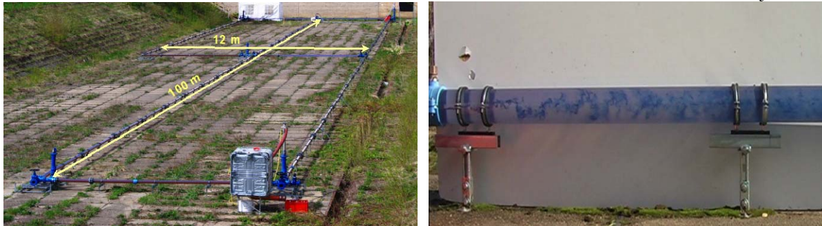
Figure 6: Test network for SMaRT-Online WDN (left); Injection experiments with a color tracer (right)
