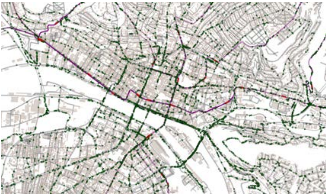
Figure 7. ESCAPE Rouen. Road network and buildings from OSM, with car (in green) and buses (in red)
