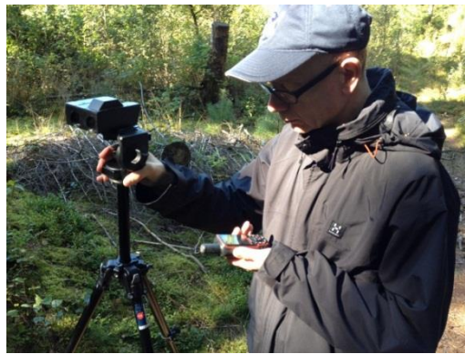
Figure 3: A participant directing the PLRF in the direction indicated by the GPS.
