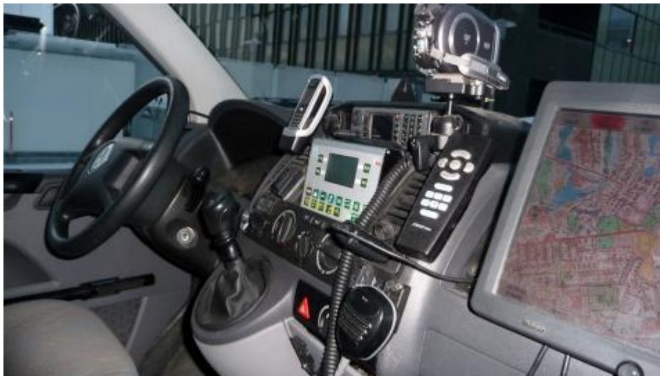
Figure 1. Interior of Finnish Police Van, showing multiple communication, computers, camera and GPS. (Image source: YLE)
