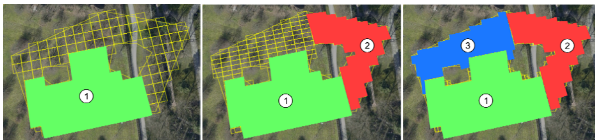
Figure 4. Partitioning to proportionally distribute workload between three unmanned aircraft.
