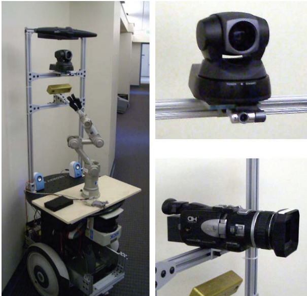
Figure 1: STAIR platform (left) includes a low-resolution peripheral camera and high-resolution PTZ camera (top-right), and alternative setup with HDV camera replacing the PTZ (bottom-right). In our experiments we mount the cameras on a standard tripod instead of using the robotic platform.
