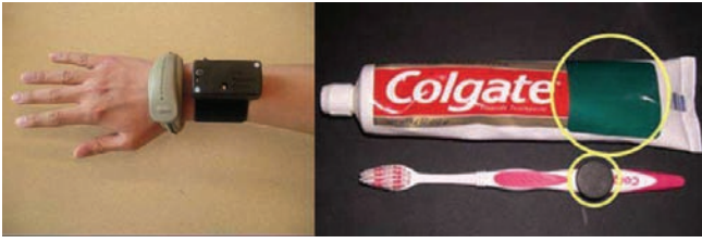
Figure 1: Sensors: iBracelet and MSP (left), RFID tagged toothbrush & paste (right), tags circled.
