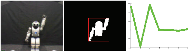
Figure 2: Aspects of visual processing. From left to right we see the source image, the foreground/background distinction, the result of object segmentation (focusing on the upper torso), and the feature signature of this posture represented as a graph connecting the seven centralised normalised moments.
