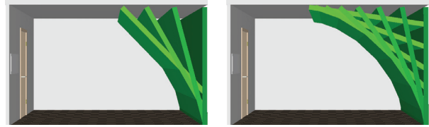
Figure 3: Motion of a garage door predicted by our non-parametric model. Left: Model after the first few observations. Right: after processing all observations.
