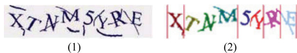
Figure 1. Segmentation. (1) A sample CAPTCHA challenge, (2) after segmentation, eight characters were identified. (Taken from [Yan and El Ahmad, 2008])
