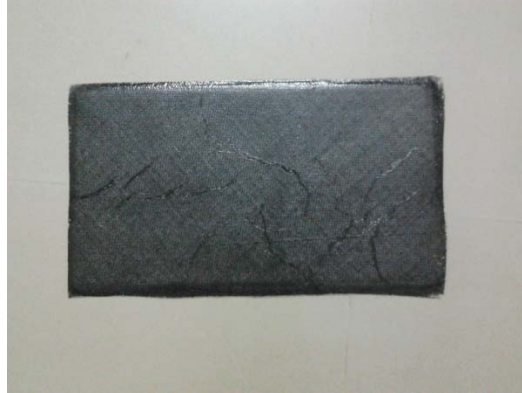
Figure 2. Glass-Epoxy laminate with graphite filler
