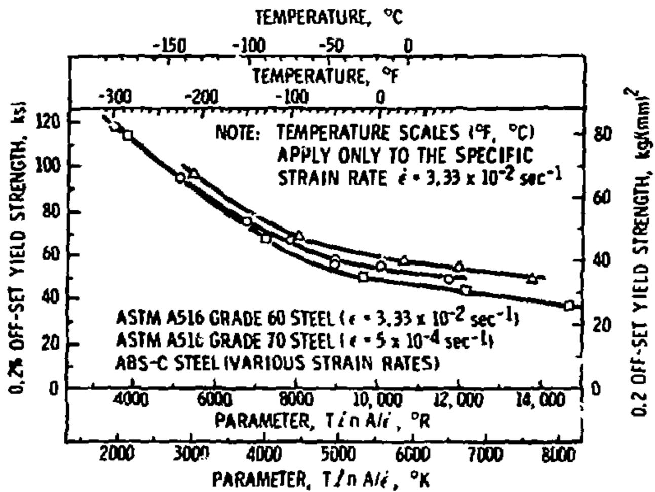
Figure 6. Rate-temperature correlation of the yield strength of ASTM A516 steel (29).
