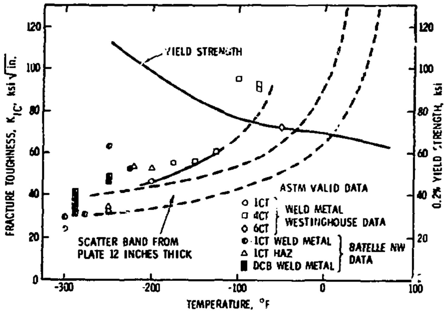
Figure 10. Temperature dependence of the weld and heat-affected zone fracture toughness of a 12 in (30.5 cm) thick weldment (Submerged Arc Process) of A533, grade B, class 1 steel plate 12 in (30.5 cm) thick; static tests - nonirradiated (31).
