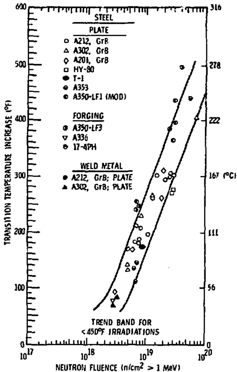
Figure 12. Increase in the transition temperature of steels resulting from irradiation at temperatures below 450° F (232° C) (33).
