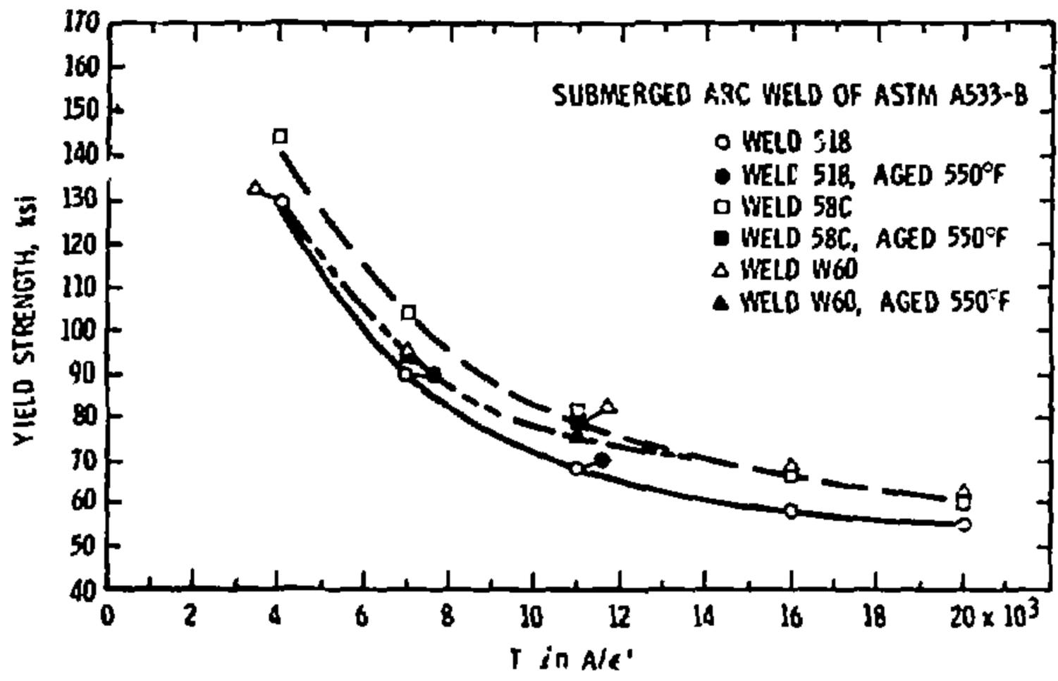
Figure 4. Rate-temperature correlation of the yield strength of three ASTM A533-B submerged-arc welds (26).
