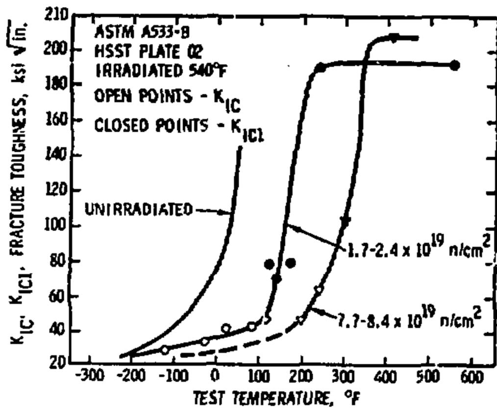
Figure 11. Irradiated and unirradiated fracture toughness as a function of temperature for ASTM A533, grade B, class 1 steel from HSST plate 02. Open data points are plane strain,  $K_{IC}$ , and closed are lower bound toughness,  $K_{IC1}$  (32).
