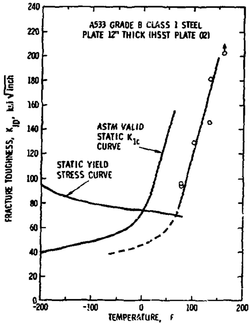
Figure 7. BTCT dynamic toughness of ASTM A533 grade B, class 1 steel for rates between  $K = 10^4$  and  $10^5 \text{ MPa}^{-3/2}/\text{sec}$  (28).
