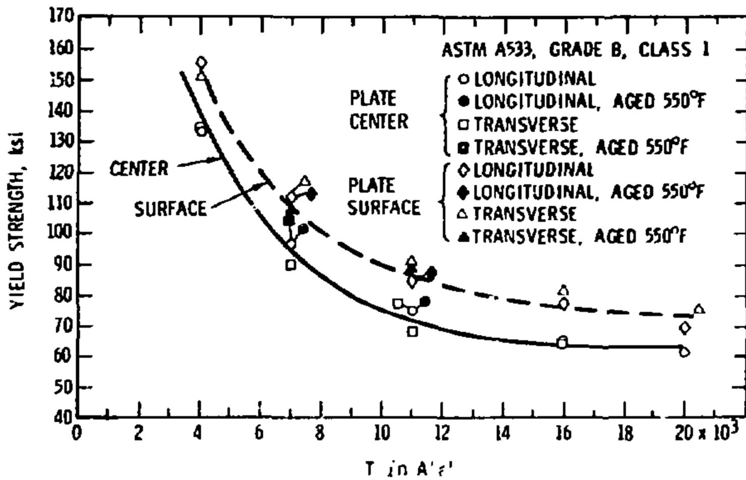
Figure 3. Rate-temperature correlation of the yield strength of ASTM A533, grade B, class 1 steel from 1/2" plate.
