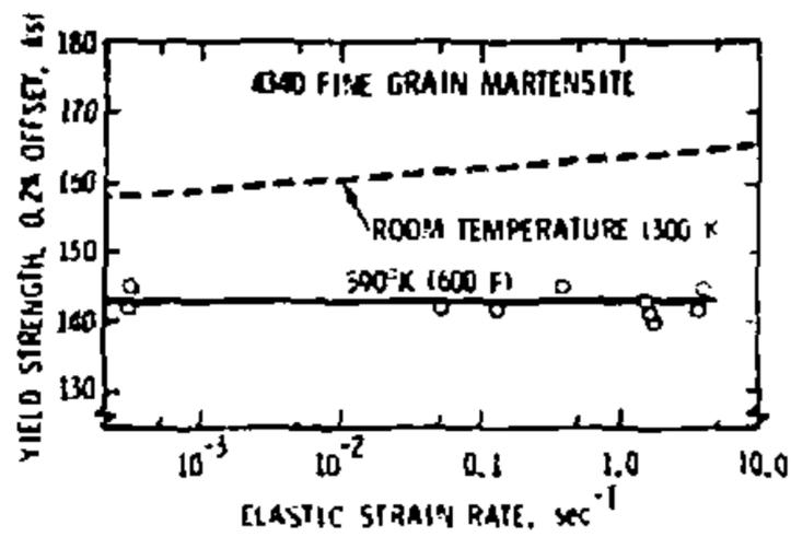
Figure 7. Yield stress versus elastic strain rate for 4340 fine grain martensite (21).
