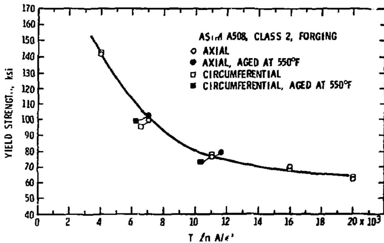
Figure 5. Room-temperature correlation of the yield strength of ASTM A508, class 2 forging (11).
