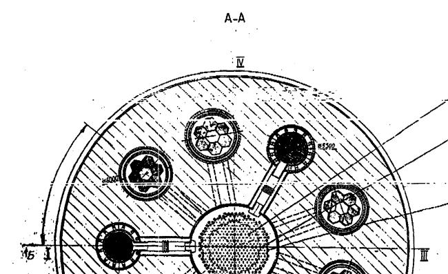
Fig.2- Acrossing Section of Reactor, 5, 6, 7 - Fuel Bundle
