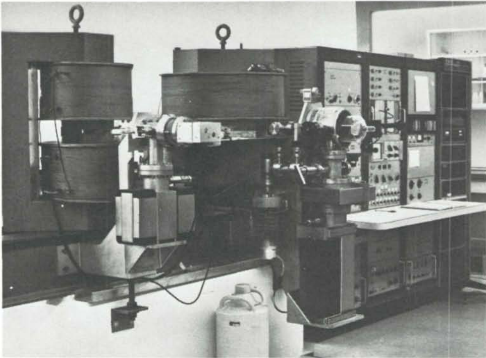
Two-stage pulse-counting mass spectrometer was specially designed for the IAEA by the Oak Ridge National Laboratory.
