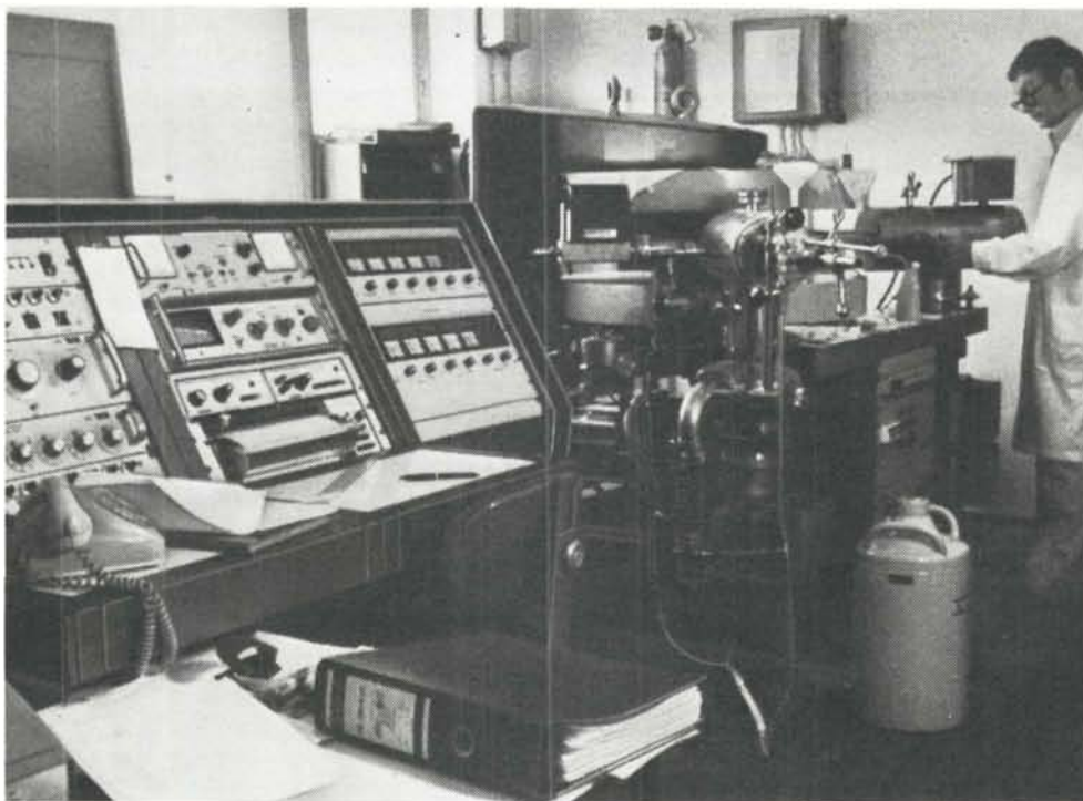
Single-stage surface ionization mass spectrometer (AVCO-type) requires 0.1 to 1 \mu\text{g} samples of plutonium or 1 to 10 \mu\text{g} of uranium.
