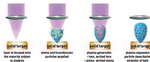
Figure 1: Schematic of LIBS plasma generation
